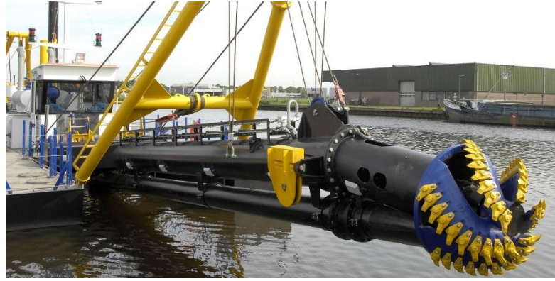
Figure 2-6: Suction pipe with cutter head
