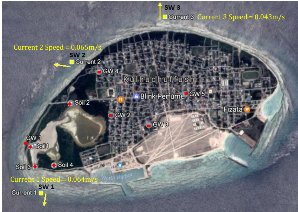
Figure 3-16: Locations showing where sea water samples (SW1-SW3), sea current measurements (Current 1-3: indicated in yellow square), ground water samples (G1-G5: indicated in red square) and soil samples (Soil 1-4: indicated in red circle) were taken. Water current (speed depicted and direction shown in arrow) GPS coordinates are given in Table below. Water current 1-3 coordinates are same as SW1-SW3 coordinates. Soil 1 coordinates are same as GW1 coordinates. Soil 2-4 GPS coordinates are 6°37'48.7"N, 73°04'10.1"E, 6°37'59.8"N, 73°03'49.9"E and 6°37'54.0"N, 73°03'50.6"E, respectively.
